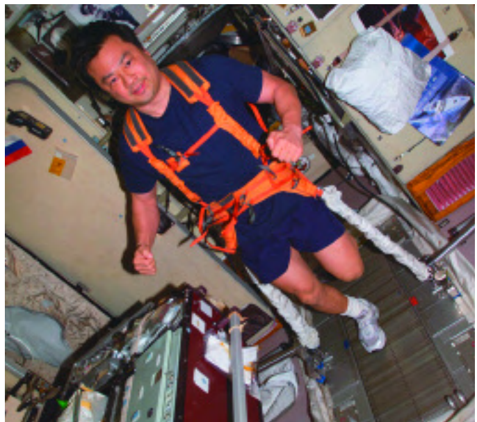
Astronaut Leroy Chiao, Expedition 10 commander and NASA ISS science officer, equipped with a bungee harness, exercises on the Treadmill Vibration Isolation System in the Zvezda Service Module of the station.
